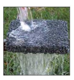
Permeable pavement looks more porous than the pavement you see on the road. You will notice if you spill a cup of water on it, the water will infiltrate right through the pavement and disappear before your eyes.
