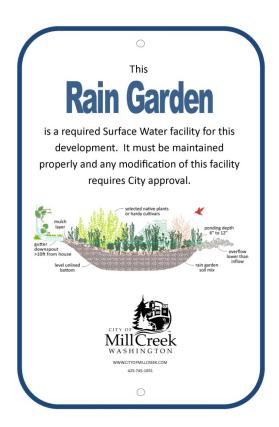
You might notice this sign at newer developments built in 2015 and after. This sign means that this is a stormwater facility that was designed to take runoff from roof drains and driveways. The water collected is designed to infiltrate into the soil.
